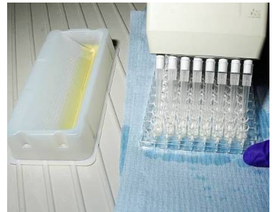
Figure 20: Add substrate and incubate at 18-25°C for 7 mins
